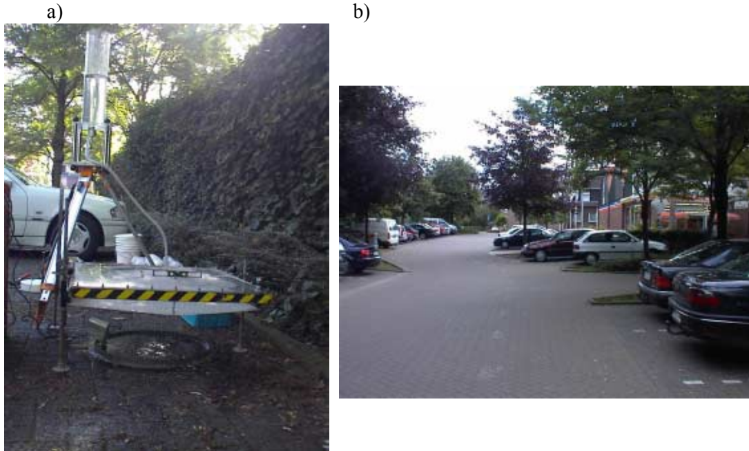
Figure 5. a) Measuring infiltration capacity with a drip-infiltrometer, b) the parking area of a supermarket in Stadtlohn
