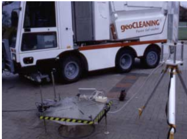
Figure 8. Measuring infiltration capacity with a drip-infiltrometer
